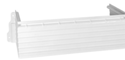
Made of fibreglass-reinforced polyester. Supplied with installation accessories. The adapter's height can be adjusted from 70 to 350 mm, by sliding the element along the outside of the window well.
