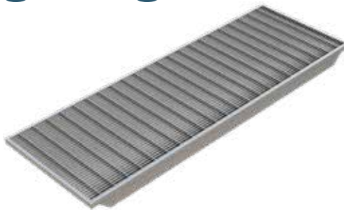
Pressure-locked grating type 20x2 - 10x2 55x11 (heelguard), with reinforcement plate, hot-dip galvanised.
