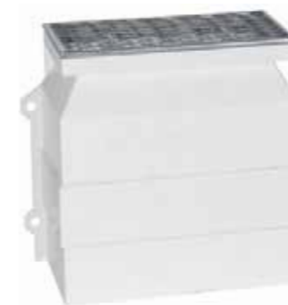
Made of fibreglass-reinforced polyester. Stackable and inclusive of fixing dowels. Easy and quick to install, they allow for creating and completing directly on-site ventilation conduits or units housing utility connections and wiring.
