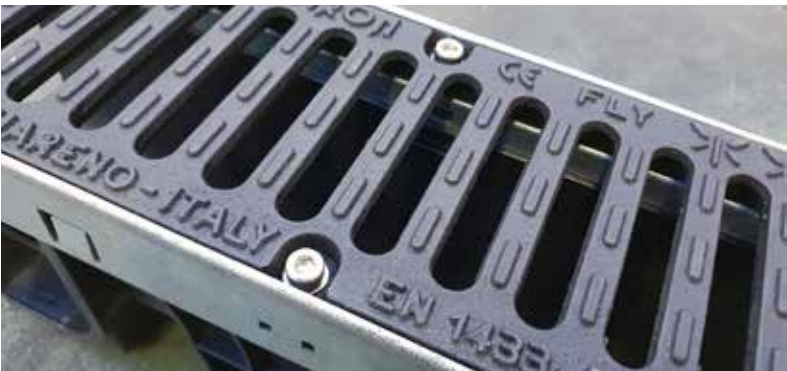
DUCTILE IRON GRATINGS SECURED TO THE CHANNEL The ductile iron gratings secured to the channel have four relief notches along their lower section which slot into the relative housings on the protective edge rail of the channel to prevent their longitudinal movement.
