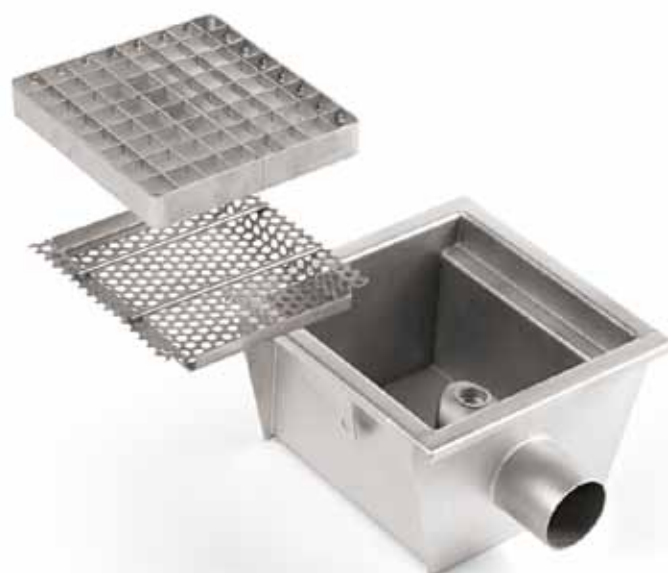
Square box horizontal drain complete with filter trap, pressure-locked pickled and polished grid, entirely made in AISI 304 stainless steel.
