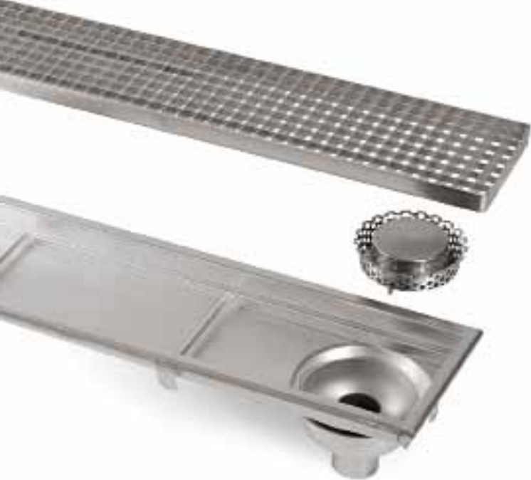
Vertical drain channel complete with filter upstream from the trap, pressure-locked pickled and polished grid, entirely made in AISI 304 stainless steel.
